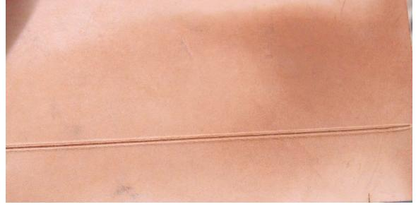
3. Use wing dividers set at bead width (1/8 inch works best in my opinion), and draw a parallel line using the cut groove as a guide.
